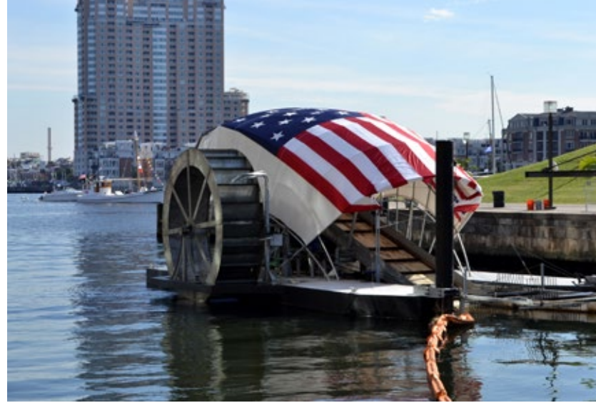
This automated device, aptly nicknamed “Mr. Trash Wheel,” collects litter in Baltimore’s harbor. Automated devices like this could supplement and expand the coverage of the skimmer boats that already operate on Chicago’s rivers.
